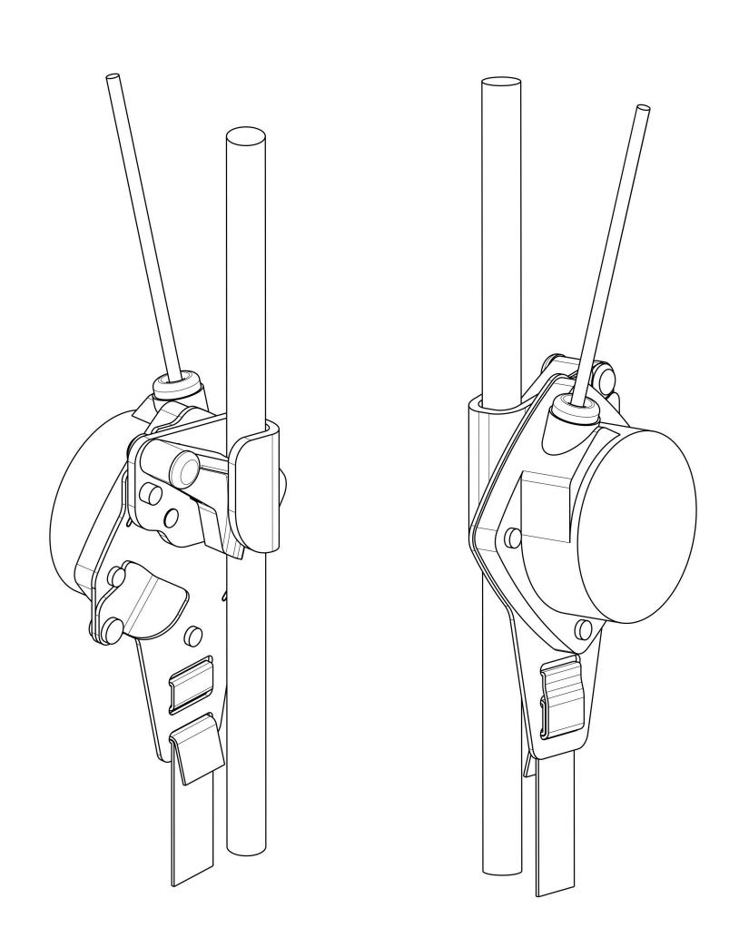
Knee ascender with integrated recoil steel spring
