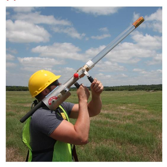
The faster you release the handle on the valve the farther the line will go. For longer distances, release the handle quicker.
