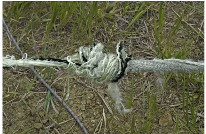
Paraloc™ Rope with 4.4 KN Tension, not yet Failed after 22 Passes on the Rope Abrasion Tester
