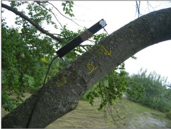
Elastometer used to determine branch stiffness
