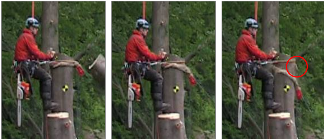
A sling may be shifted over a small stub when put under tension
