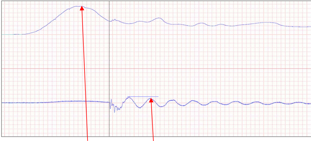
Figure 8.13 Load and fibre strain curves for log dropped from approx. 5 m height in field tests (drop no. 20)
