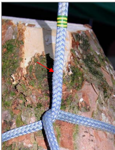
Slippage through a supplementary Half Hitch
