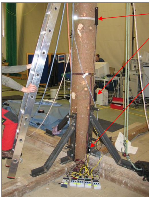
Set up of Tree-Statics instruments
