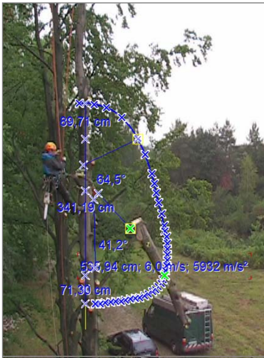
Trajectories of a log and a crown section*
