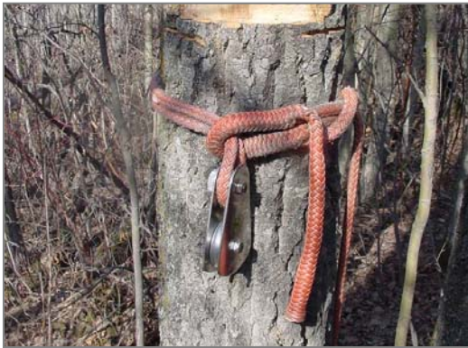
Loopie sling with arborist block (correct configuration)*
