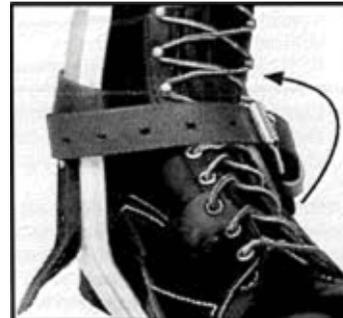
Step each foot into the climbers with gaffs on the instep side of the foot. The longest curvature of the cuff designates the front of each climber.
