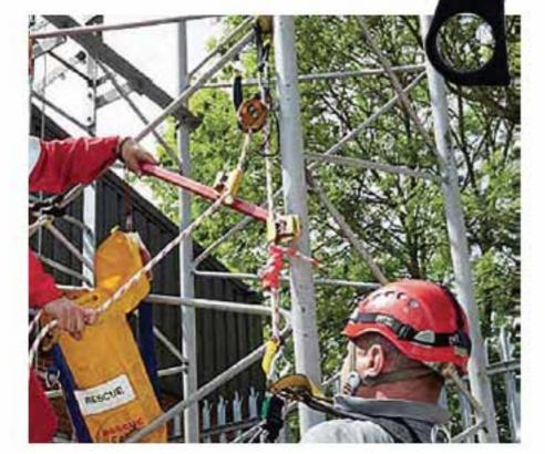
the two ropes and gain much distance whereas the version in this photo can gain several inches more per stroke but it's still a rather ineffectual way of doing things. In this particular instance, a mini pulley system in a bag might be easier to carry for a casualty pick off rescue where you only need to de-
